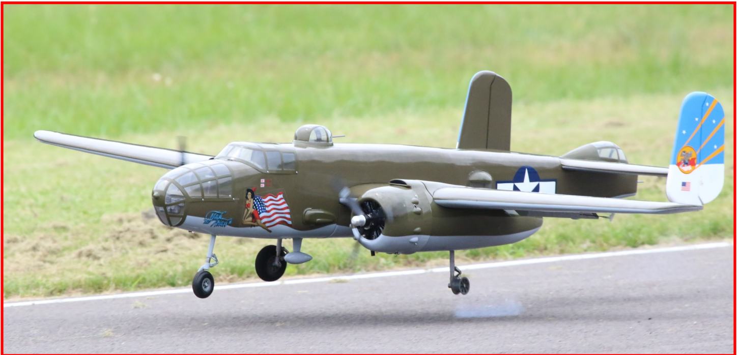
Dramatic shot of Jaime's B-25 making a landing at the Warbird Fly-In — missing the left main gear tire that came apart upon the first touch down just before this shot was taken.
